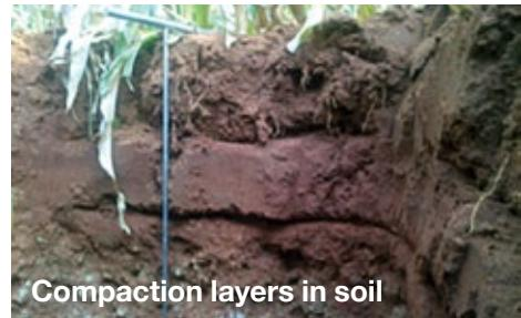
Compaction layers in soil
